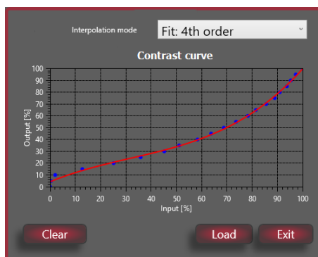
Figure 3-62 Contrast correction curve using 4th order interpolation
