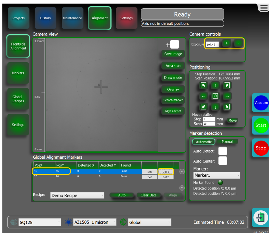
Figure 3-137 Going towards marker position
