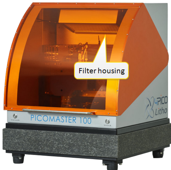
Figure 4-23 HEPA filter location
