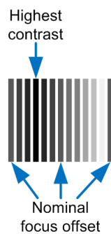
Figure 3-71 Best focus determination by microscope
