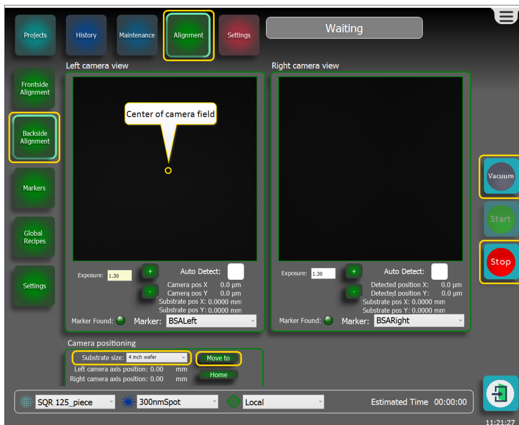
Figure 3-112 Searching the backside alignment markers
