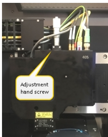
Figure 3-14 Turning the manual z-adjustment screw
